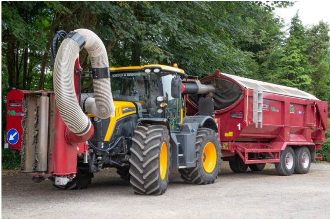
Picture 8: Lincolnshire Verge Harvesting (LVH) Ltd self- designed ‘wrap around cut and collect harvester.
