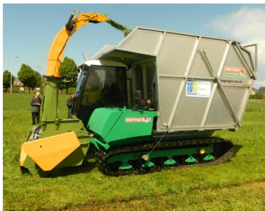
Picture 7: Self-propelled Log Logic Soft Track 15 low ground pressure wetland biomass harvester
